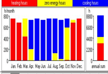
As mentioned above, that the double-glazing windows with aluminum frame are the most advantageous of the lot we have considered, the above graph will give us a better understanding to that statement. It is evident from the graph that both the heating load and the cooling load have reduced by a factor of 2, which is a considerable amount considering the peak summers weather conditions in New Delhi.
