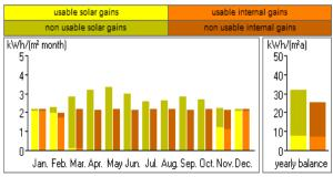
From the above graph it is very clear that the single glazing windows is used will result in the rise of the cooling load especially in the months of May, June and July, that is, during peak summer. In the second figure, we can see that the useful solar gain and the transmission losses which will be there when the single glazing window is used in our building.
