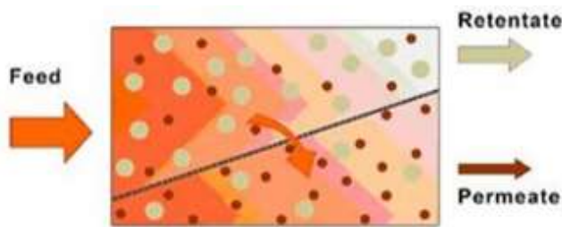
Fig 1: Schematic model of the membrane functioning
