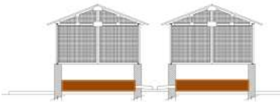
Figure 10 step four water sprinkling has been stopped and wastage is left to get dry.
