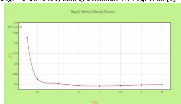
Fig. - 4 C_d vs h/c of calculated data for rear wing of car.
