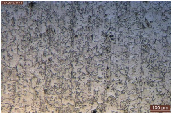
Figure 4 7: Optical Microscope of Nitrided FSS for 24 Hours in Ammonia Environment at 600 (100x Magnification)
