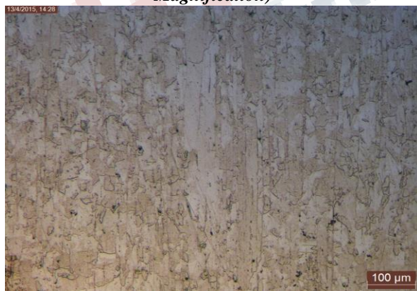
Figure 4 3: Optical Microscope of Nitrided FSS for 2 Hours in Ammonia Environment at 600 (100x Magnification)
