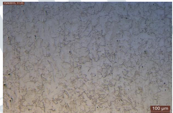
Figure 4 5: Optical Microscope of Nitrided FSS for 8 Hours in Ammonia Environment at 600 (100x Magnification)
