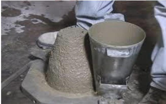
**TABLE:6 RESULTS FOR SLUMP CONE TEST FOR QUARRY DUST MIX CONCRETE**
