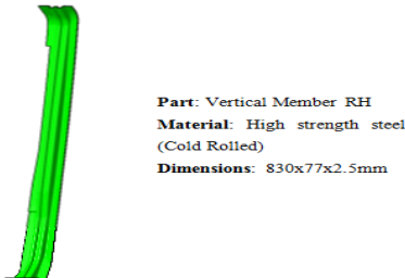
Figure 8: Vertical member at RH Side and LH Side at the Rear wall
