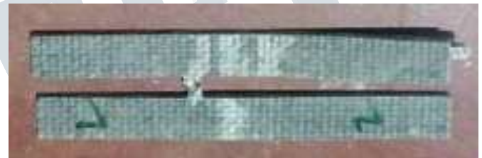
Fig 2: Flexural test specimens of 1% & 1.5% of graphene
