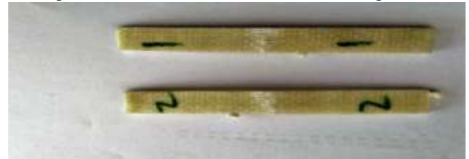
Fig 1. Flexural test specimens of 0% & 0.5% of graphene
