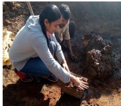
**Fig. 5. Moulding of green Clay Mixture**
