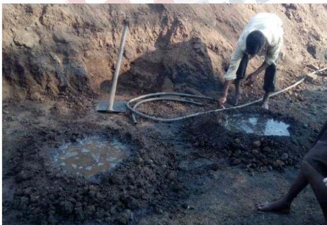
**Fig. 2. Preparation of mud in mud-pool**
