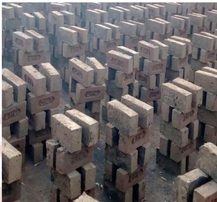
**Fig. 7. Sun drying of Bricks**
