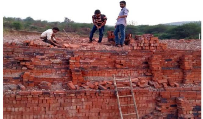
**Fig. 9. Removal of burnt bricks from kiln**
