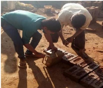
**Fig. 6. Sorting of moulded clay over earthen floor**
