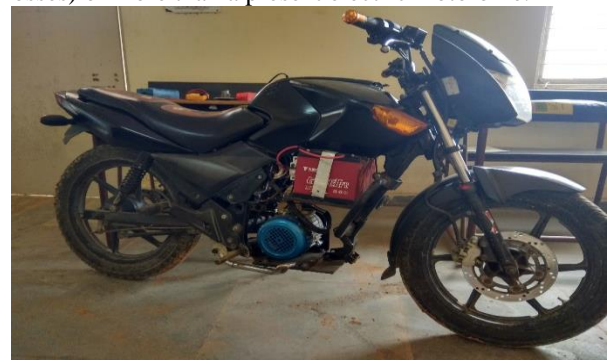
Figure: Retrofitting of Electric Drive train on an I.C. Engine bike (TVS Flame).
