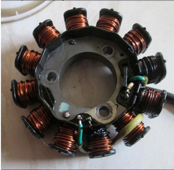
Figure: Alternator, capable of giving peak charging output of 300Watts
