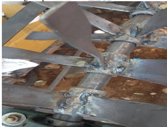
Fig.9. The Blade and Hub Assembly held on the
