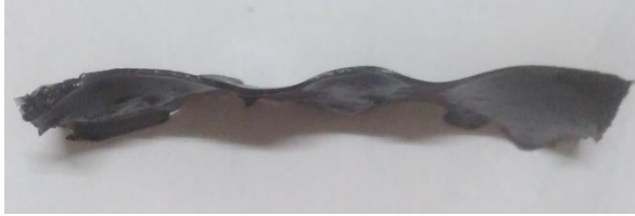
Fig. 2.4 SMP sample after heating exhibits shape memory effect
