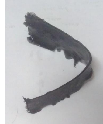
Fig. 2.3 SMP sample after un-loading
