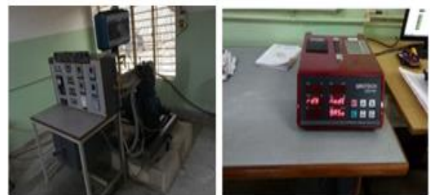
Figure 4: Diesel Engine Test Rig Figure 5: Exhaust Gas Analyzer
