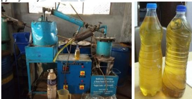
Figure 3: Extraction of plastic oil by pyrolysis process
