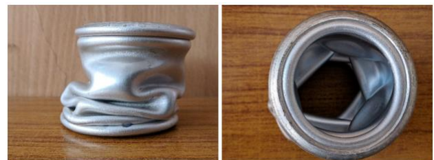
Figure. 12 Dynamic test specimens under interrupted loading of annealed tubes
