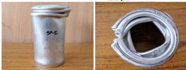
Figure. 10 Dynamic test specimens under interrupted loading of as received tubes
