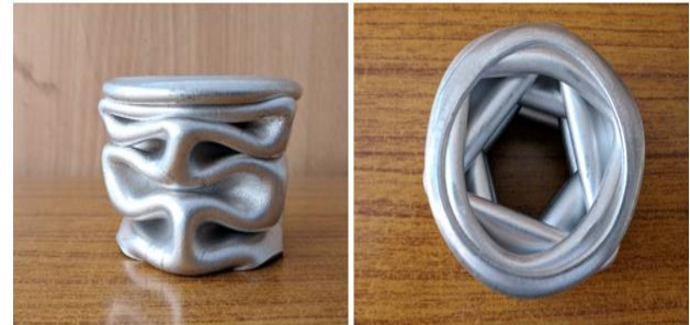
Figure. 14 Quasi-static test specimens for intermittently annealed interrupted loading
