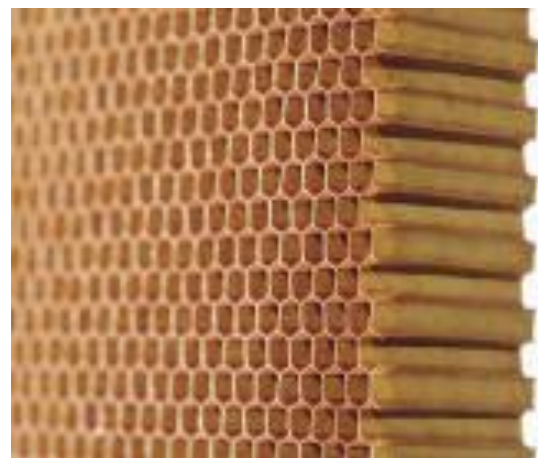
Fig-1.2: Explored view of aramid honeycomb structure
