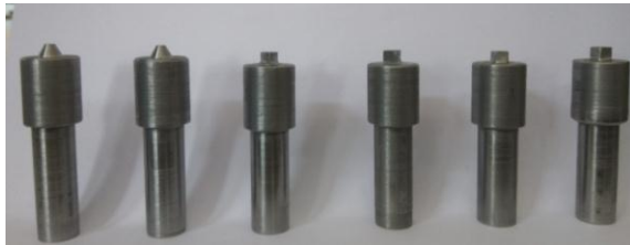
Fig 2.1 Conical, Square and Triangular tools
