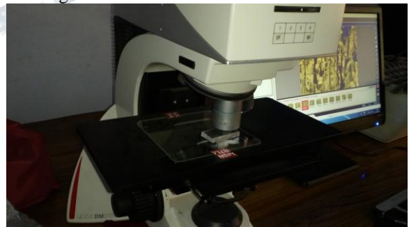
Fig 2.3 Tool Maker's Microscope with sampled specimen
