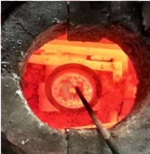
Figure No. 1 Stir casting of specimen
