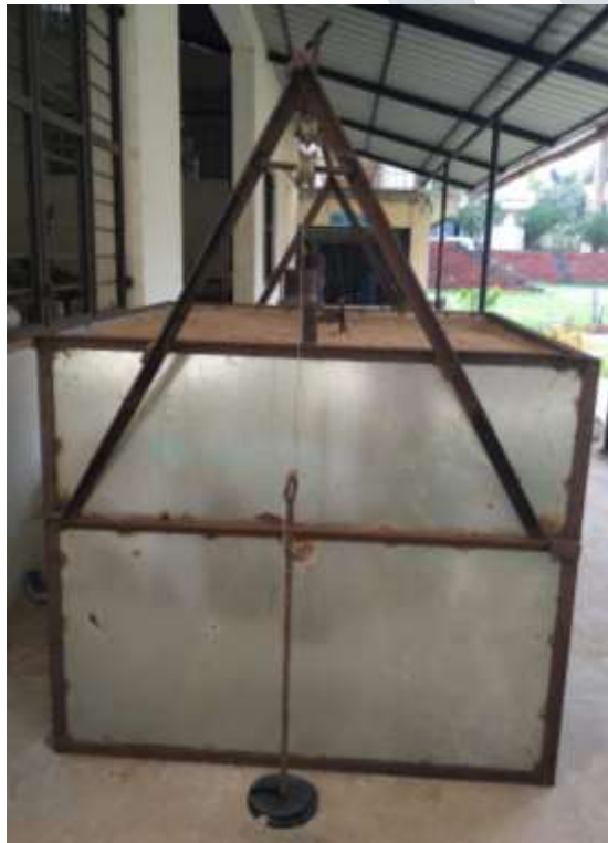
Fig. 5 Pullout loading arrangement
