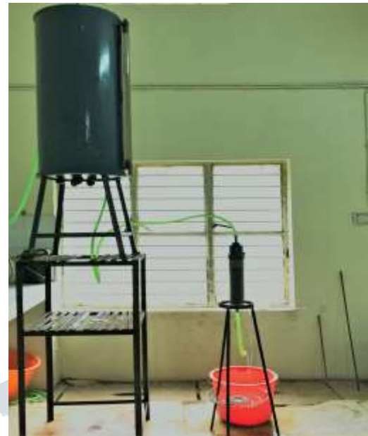
Fig. 3 Rigid- wall column erosion test apparatus
