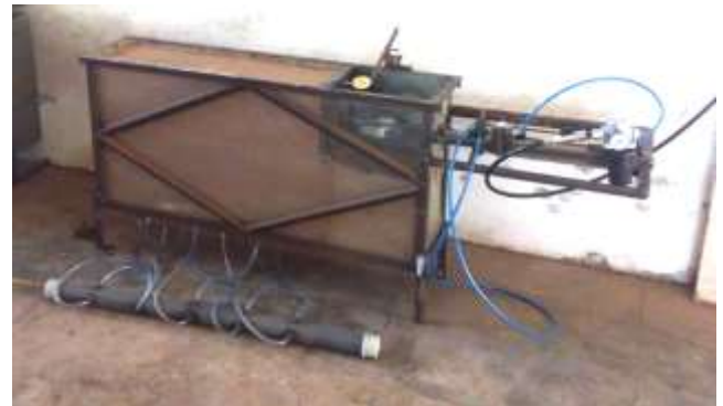
Fig.2. Pneumatic set up for lateral loading
