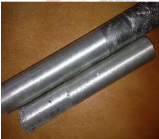
Fig.4 Finished casting after rough turning
