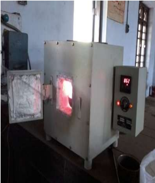
FIG2. Preheating of Graphite at 9000C
