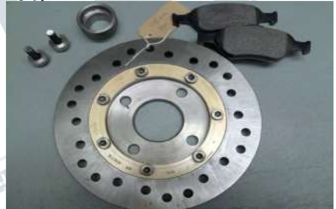
Fig 5. Prototype brake disc
