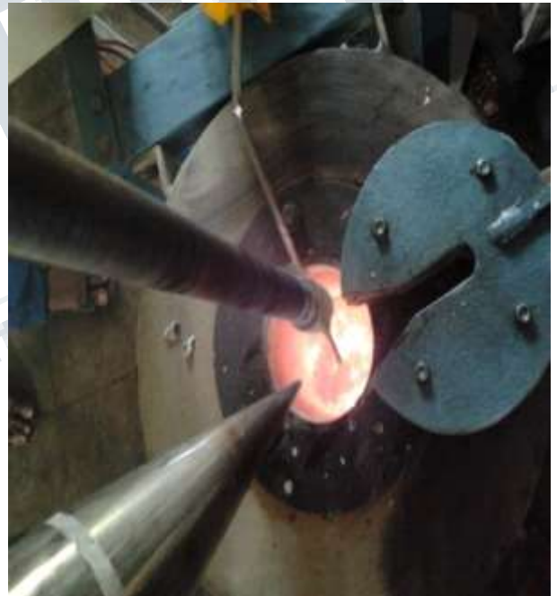
Fig.1. Molten LM6 in the furnace at 7500C
