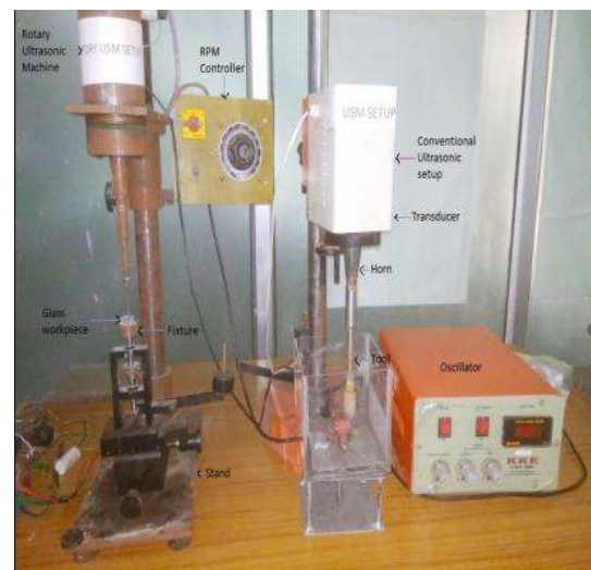
Fig.2: Setup of rotary ultrasonic machining
