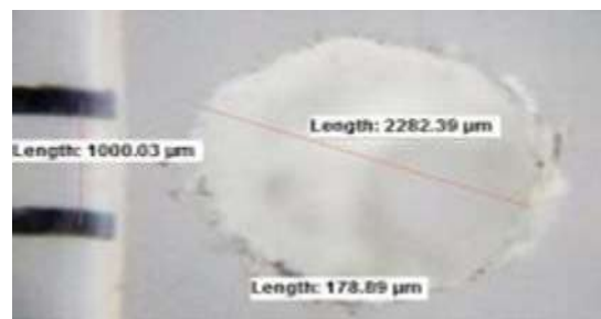
Fig 3: Overcut by rotary USM at 1000 rpm and measurement of hole diameter with optical zoom
