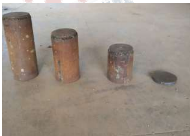
Fig. 3 Skirted Circular Footing
