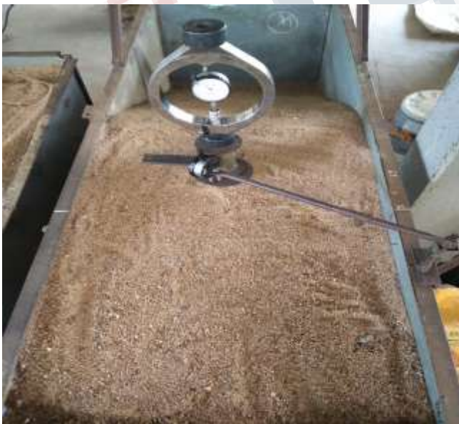
Fig. 5 Axial loading set up
