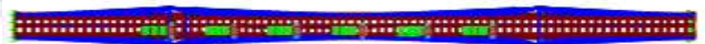
Fig 5.1- 70 R wheeled vehicle moving from one end to the other end of the bridge in lane one of bridge
