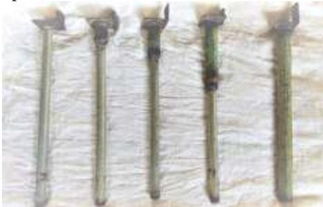
**Fig. 2 Step tapered piles**
