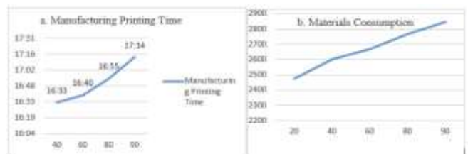
Figure 5: Effect of infill density: (a) Graph Between Manufacturing Printing Time with Infill Density (b) Materials Consumptions with Infill Density
