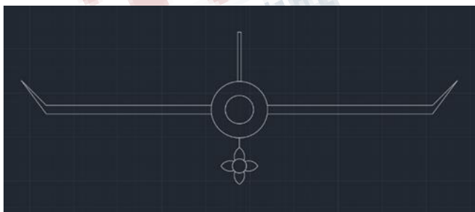
Figure 6: Final AutoCAD Design (Front View)
