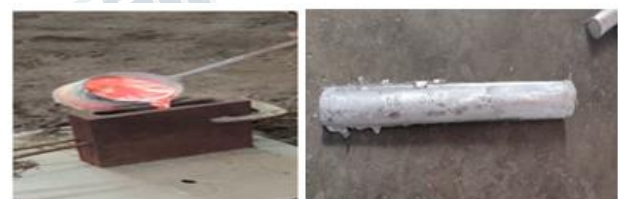
(a) Pouring molten metal (b) Casted product
