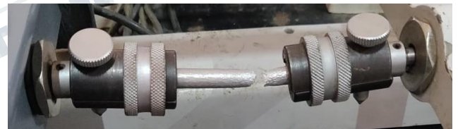
Fig 4.3: Tensile specimen broken
