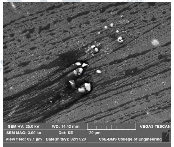
Figure 5.4: The distribution of Al and 9% weight composition of TiO 2 composite sample.
