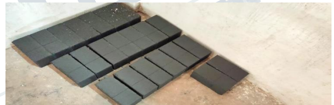
Fig 4.31 Bagasse Ash bricks
