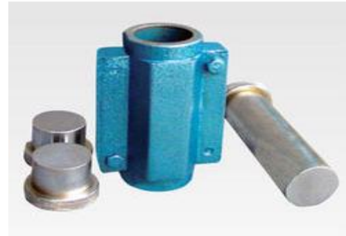
Fig 4.1.1: Split mould 38mm dia x 76mm long
