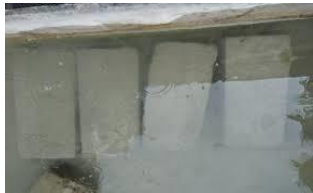
Fig 3. Water Absorption test
