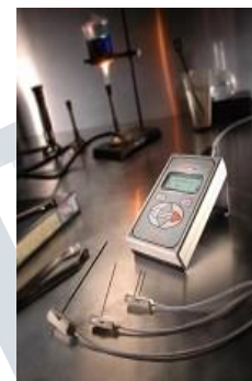
Fig 7. KD2 pro instrument for thermal conductivity
