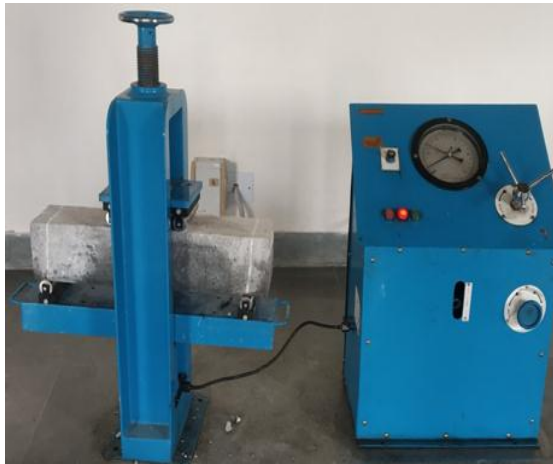
Fig3: Flexure Testing Machine
