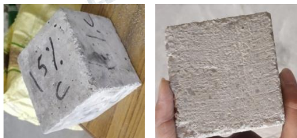
FIG 3.4.3: a) Specimen without abrasion test b) Specimen after abrasion test
