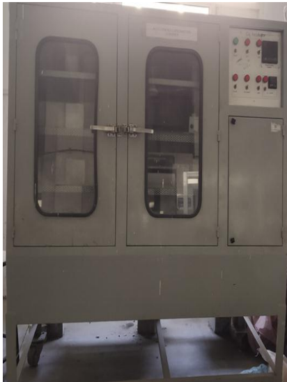
Fig6 :Accelerated Carbonation Chamber
