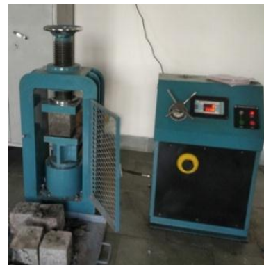
Fig2:Compression Testing Machine
