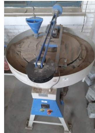
Fig4: Abrasion Testing Machine
