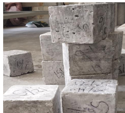
Fig5 :Specimens Coated with parrafin wax
