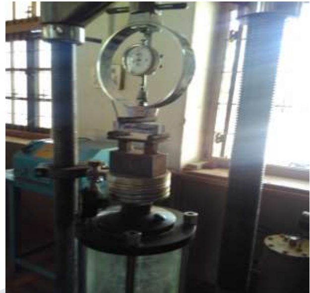
Figure 2. Loading frame for 3 point bending test
