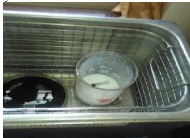
Figure 1. Ultrasonic Bath Dispersion of MWCNTs and nano- Al_2O_3
