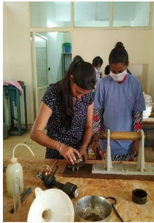
Fig. 5 Preparation of UCS samples for contaminated soil
