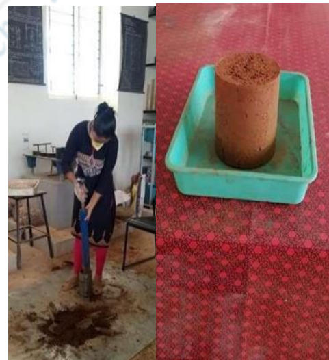
Figs. 3 and 4 Standard Proctor test for contaminated soil
