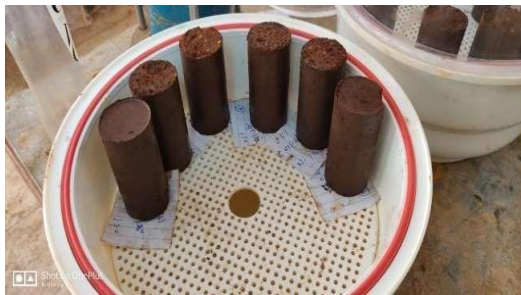
Fig. 6 UCS prepared samples under curing
