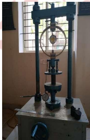
Fig. 7 Unconfined Compression Testing
