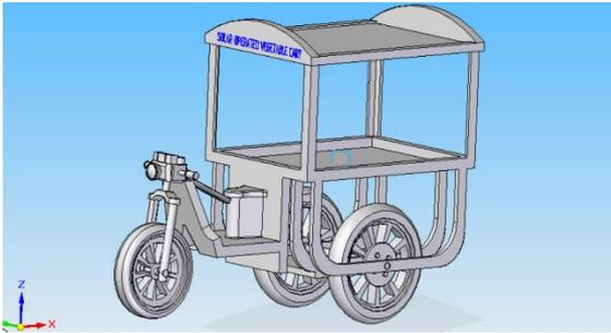
Figure 8: Conceptual Proposed Design for Solar Operated Vegetable Cart.
