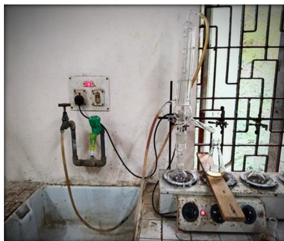
Fig. 7- Macro-Kjeldahl method- (Total Kjeldahl Nitrogen Test)
