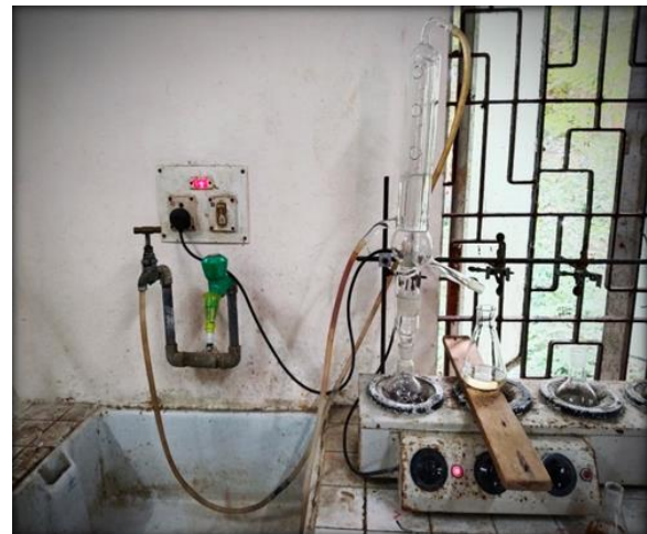
Fig. 7- Macro-Kjeldahl method- (Total Kjeldahl Nitrogen Test)
