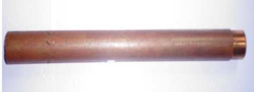
Fig. 1: (b) Circular copper electrode tool of 15 mm diameter
