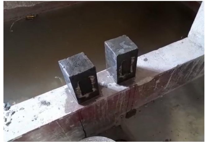
Fig. 5 – Take out bricks from water after 24 hours
