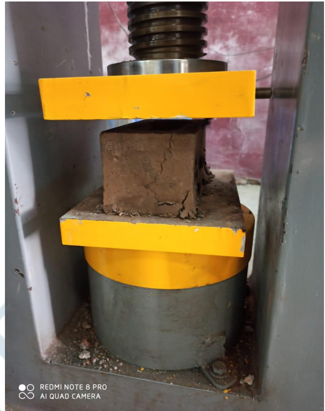
Fig. 3 – Compressive strength testing of plastic brick
