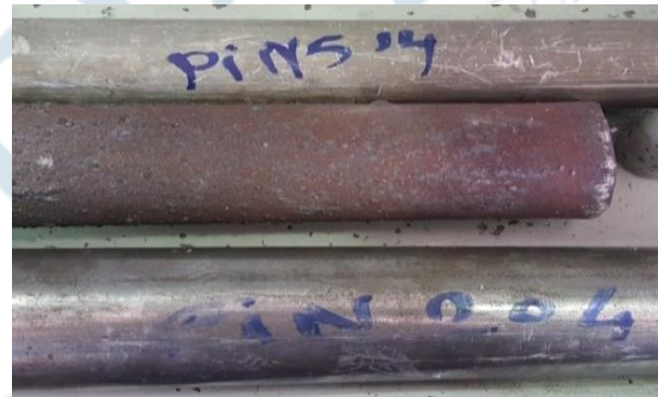
Fig.(1) Steel (pin 204), Al (pin 514), Cast iron (alloy) samples
