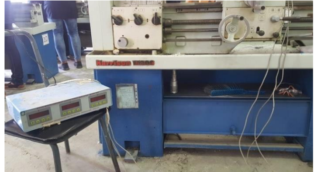
Fig.(4) high speed lathe Marrison (M 300) with dynamometer
