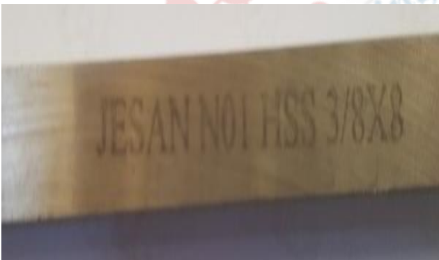
Fig.(3). HSS (3/8x8) cutting tools
