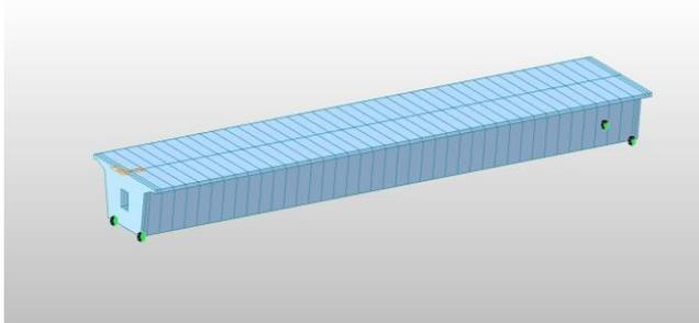
**Figure 4:** 40m Single Span PSC Box Girder
