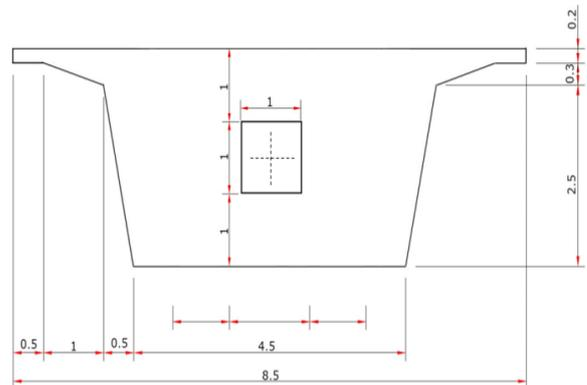
**Figure 2: Diaphragm Section**
