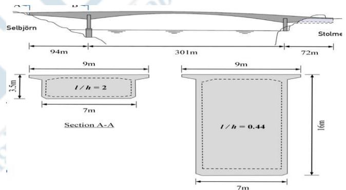
**Figure 1:** Box Girder Diaphragm Segment
