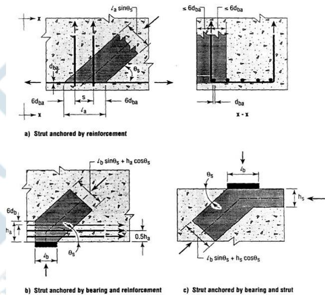
**Figure 8:** Anchorage conditions on effective cross-sectional area of strut (AASHTO LRFD)
