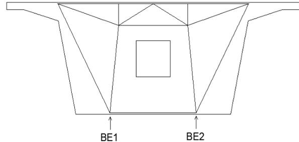
**Figure 5:** Truss Model for Diaphragm
