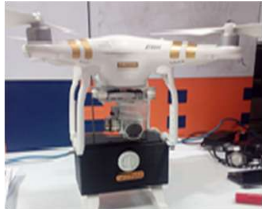
Figure 9: Integration of the designed embedded circuit enclosure box with the Quad copter
