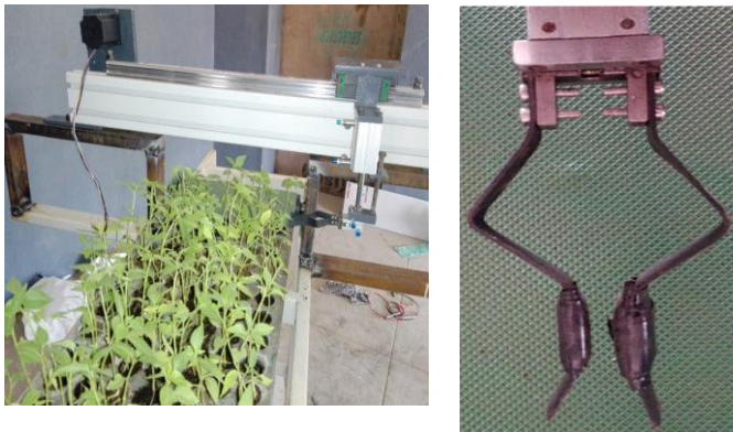
Fig. 3 Development of an experimental set up for an automatic transplanting mechanism
