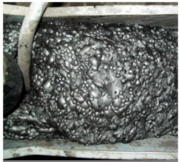
Image of froth at the onset of the run (t = 0 min)
