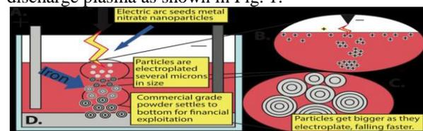
**Figure 1: Schematic of aqueous arc plasma synthesis setup to make micro-particles.**
