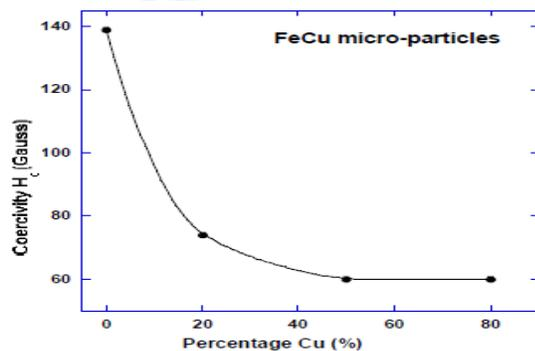
Figure 4: H<sub>c</sub> vs %Cu in FeCu micro-particles.
