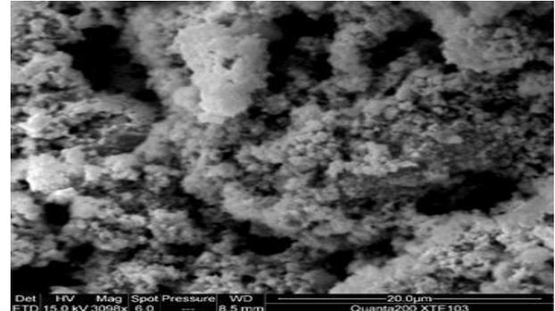
Figure 2: SEM viewgraph of FeCu micro-particles
