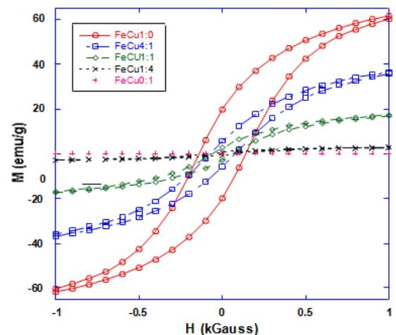
Figure 3: Magnetization M of FeCu micro-particles with applied magnetic field H.
