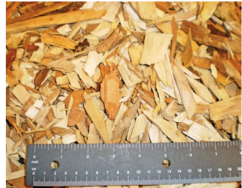
Fig.2. Woodchips commonly used in woodchip bioreactors
