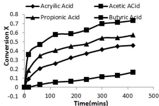
**Fig. 2 Effect of different type of mono-carboxylic acids used in the esterification reaction with ethanol. Reaction condition: RE/A = 1; HCl as catalyst; temperature = 333.15K.**
