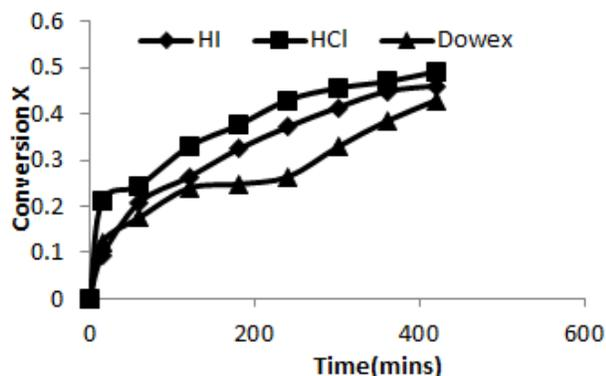
**Fig.1 Effect of the different types of catalyst used for the esterification reaction. Reaction condition: RE/A = 1; temperature = 333.15K.**
