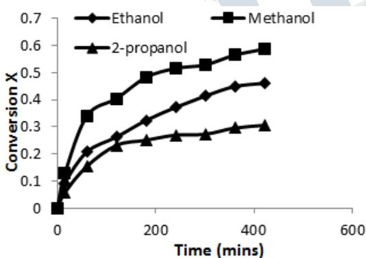
**Fig.3 Effect of varying the type of alcohols used. Reaction condition: RE/A = 1; HCl as catalyst; temperature = 333.15 K.**
