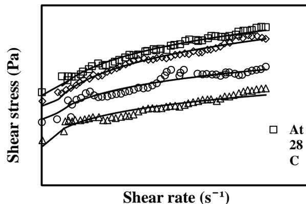
**Fig. 3** Steady flow behavior of water clover leave puree (blanched) at selected temperatures
