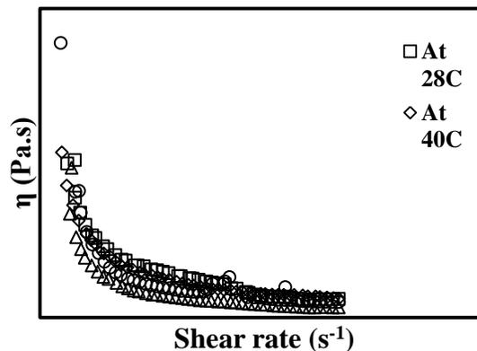
**Fig. 4 Influence of temperature on steady shear viscosity of blanched water clover leaves puree**
