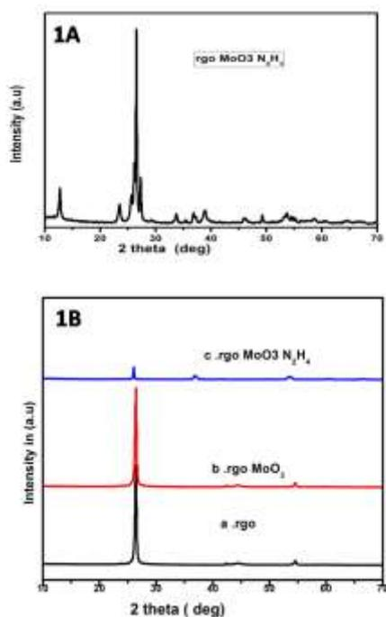
**Fig.1(A) X-ray diffraction patterns of RGO/ $\text{MoO}_3$  and in Fig 1 (B) pattern (a) for RGO, (b) for pure  $\text{MoO}_3$  and (c) for RGO/ $\text{MoO}_3$ .**
