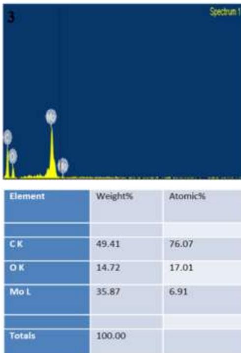
**Fig. 3 EDX pattern of the compound and Table 1 the elemental composition derived from EDX analysis.**
