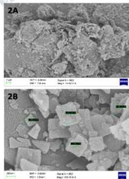
**Fig.2 FE-SEM images, (A) and (B) of RGO/  $\text{MoO}_3$  samples at different magnifications.**
