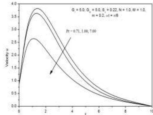
Fig. 4: Effect of  $P_r$  on the primary velocity  $u$ .
