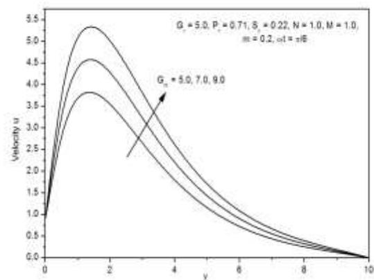
Fig. 16: Effect of  $G_m$  on the primary velocity  $u$ .
