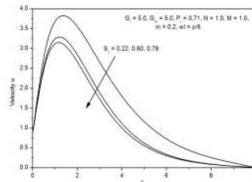
Fig. 6: Effect of  $S_c$  on the primary velocity  $u$ .
