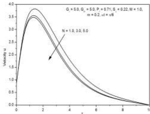
**Fig. 8:** Effect of  $N$  on the primary velocity  $u$ .
