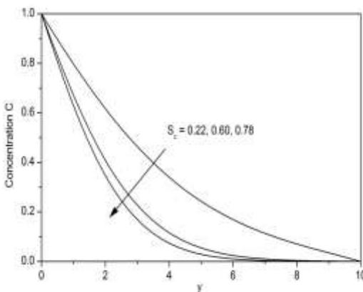
Fig. 3: Effect of  $S_c$  on the concentration distribution.
