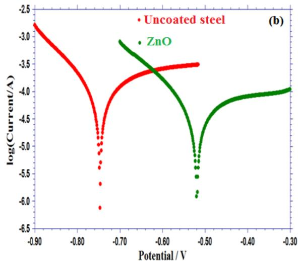
Figure 4 Tafel plots in (a) 0.1M HCl and (b) 3.5% NaCl solution after immersion ZnO nanoparticles
