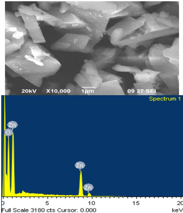
Figure 3 SEM image and EDS spectrum of ZnO nanoparticles
