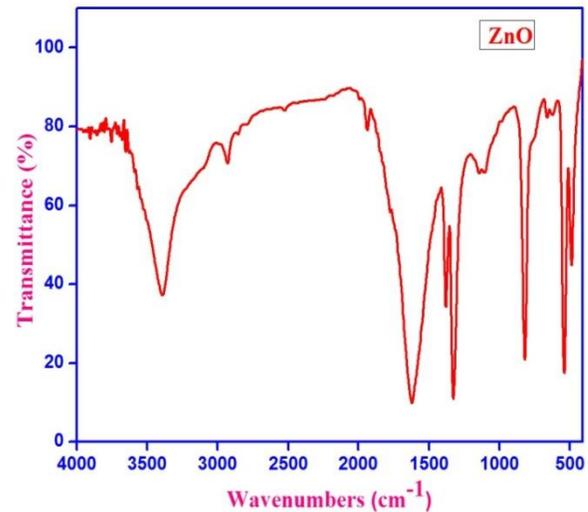
**Fig 1: FT-IR spectrum of ZnO nanoparticles**
