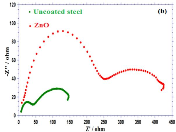
Figure 4 Nyquist plots in (a) 0.1M HCl and (b) 3.5% NaCl solution after immersion ZnO nanoparticles
