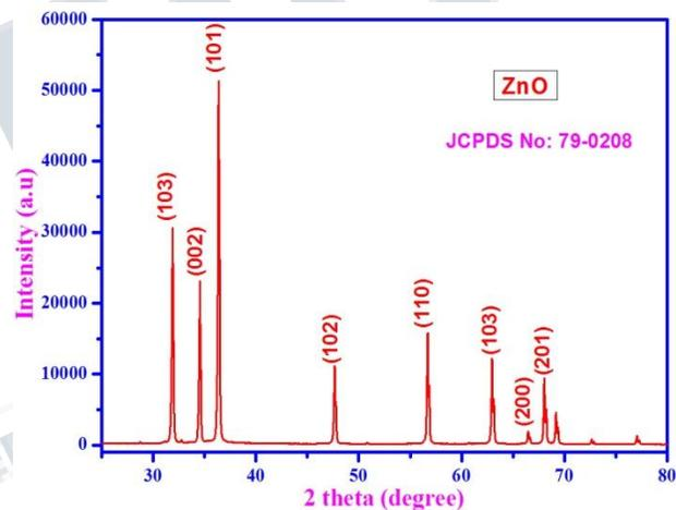
**Fig 2: XRD spectrum of ZnO nanoparticles**
